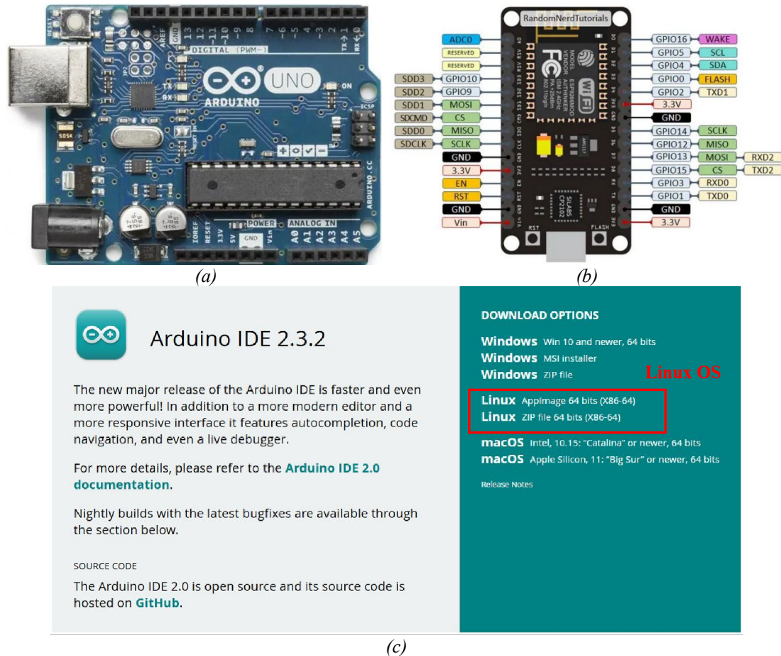
Figure 1: Simple open-source hardware that can be developed under the Linux operating system. (a) Arduino Development Board. (b) WiFi Module. (c) Arduino IDE Download Options.
