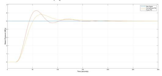
Figure 7: Closed-loop step responses of conventional PID and fuzzy PID.
