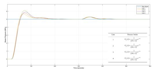
Figure 9: Closed-loop step responses of fuzzy PID with different parameters.
