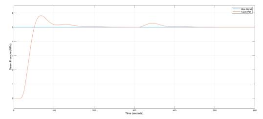
Figure 8: Closed-loop step responses of fuzzy PID with disturbance applied.
