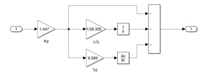
Figure 3: Conventional PID controller of the combustion control system.
