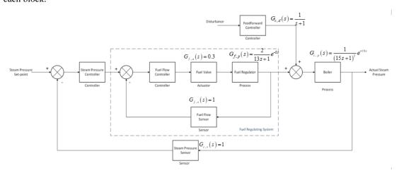
Figure 1: Block diagram and transfer functions of the combustion control system.
