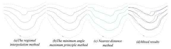
Figure 11: Contour comparison of interpolation in areas with low similarity.
