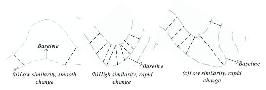
Figure 4: Contour area partition after baseline exchange.
