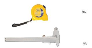
(a)- tape (b)- Vernier caliper
