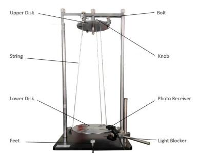
Figure 5: DH4601 The three-string torsional pendulum
