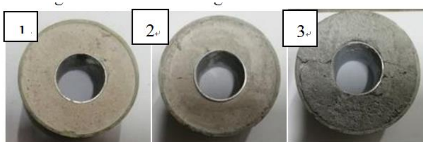
(1) Crushing morphology at 0.6MPa (2) Crushing morphology at 0.7Mpa (3) Crushing morphology at 0.8Mpa
