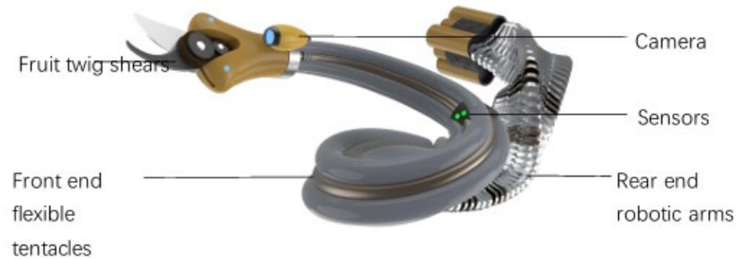
Figure 8: Structure of the bionic octopus tentacle robotic arm
