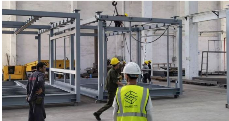
Figure 4: Production diagram of modular structure system
