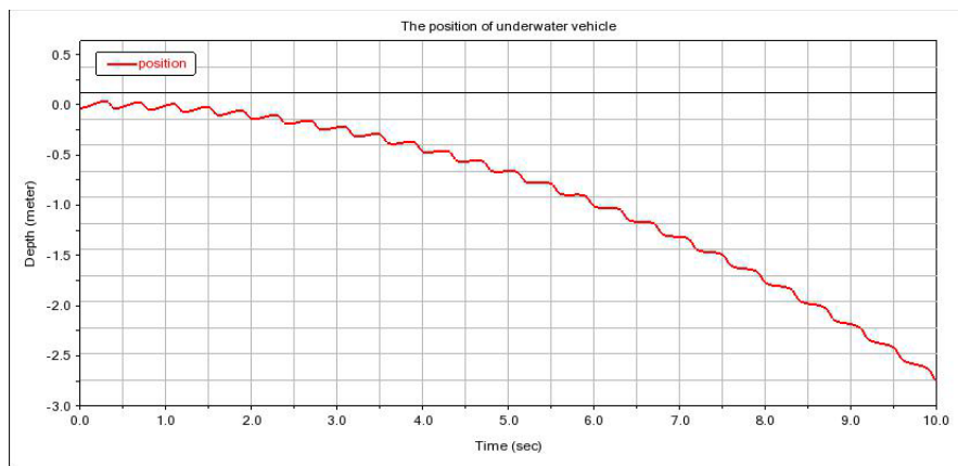
Figure 15: The change of the position of the center of mass in the first 10 seconds when harmonic motion.
