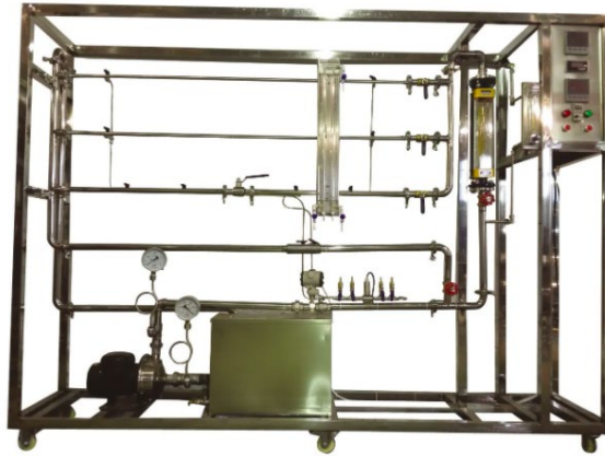
Figure 1: Physical picture of comprehensive experimental device for flow process.
