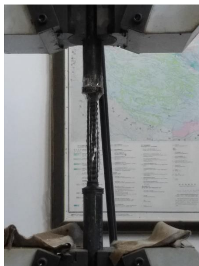
(a) Breakage during the Test Process
