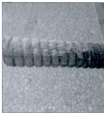
(a) Internal Thread Damage of GFRP Nuts (b) Surface Damage of GFRP Tendons
