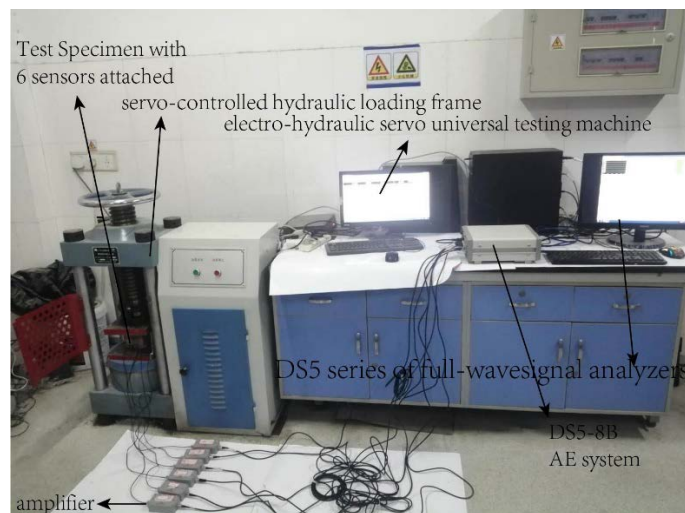
Figure. 2 Photograph showing actual test setup
