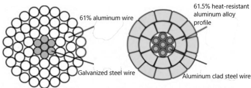
Figure 2: Conductor structure comparison
