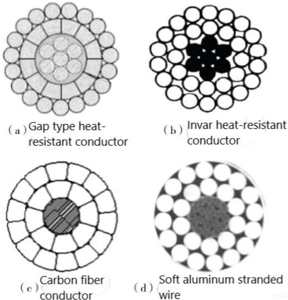
Figure 3: Cross sections of several heat-resistant conductors
