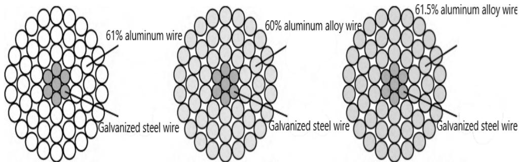
Figure 1: Conductor Structure Comparison
