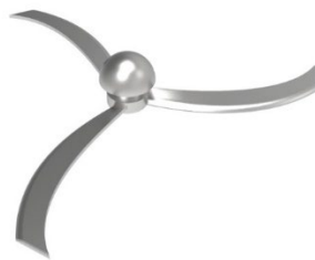
Figure 8: Schematic diagram of the arc-shaped inclined scraper structure
