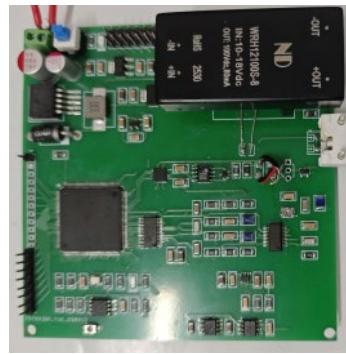
Figure 13 Physical image of FPGA circuit board
