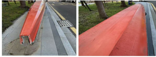
Figure 1: Biofouling on a dragon boat hull underside.
