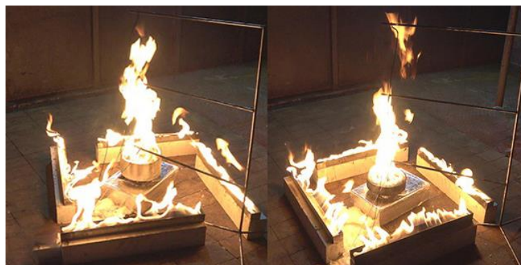
Figure 3: Typical rotation fire observed in experiments. Left: rotation fire for the pan's height is H = 5\text{cm} ; right: rotation fire for the pan's height is H = 10\text{cm}
