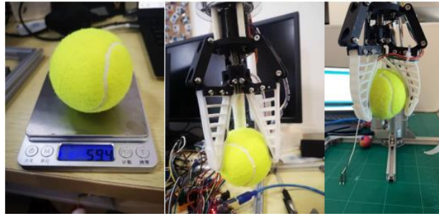
Figure 6: Gripping test tennis ball, weight 59.4g, diameter 6.3cm, 90 hardness gripping success, 30 hardness gripping success.
