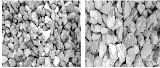
Figure 2: Recycled aggregate particle size 10-16mm and 16-20mm.
