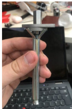
Figure 12: Visual representation of how yaw system works with concrete flooring bold at a substitute axle.
