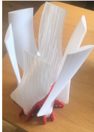
Figure 9: Folding hub with blades in closed position.
