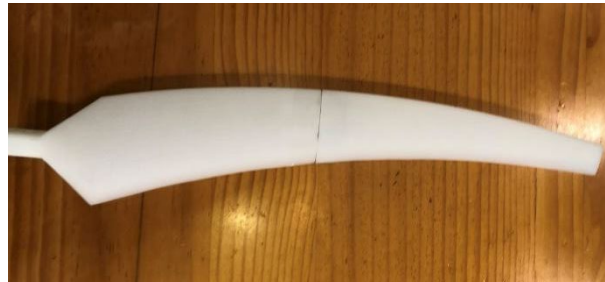
Figure 6: Second blade iteration resin printed.
