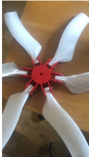
Figure 8: Folding hub most recent iteration with blades deployed.
