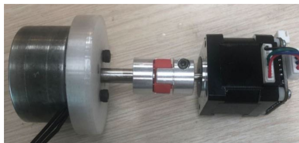
Figure 3: 60-watt generator with a stepper motor connected to a program on the computer that can vary its rotation.
