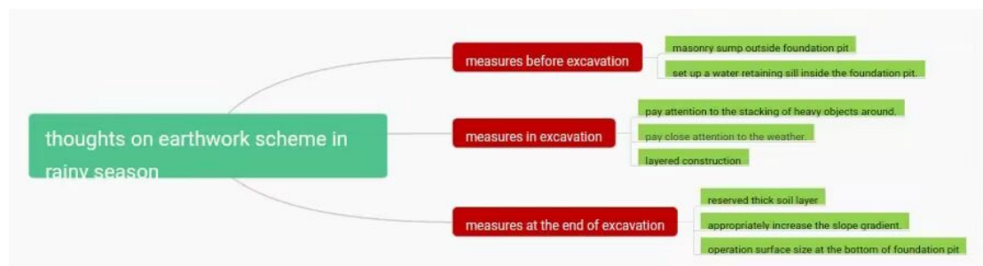
Figure 5 Idea diagram of earthwork measures
