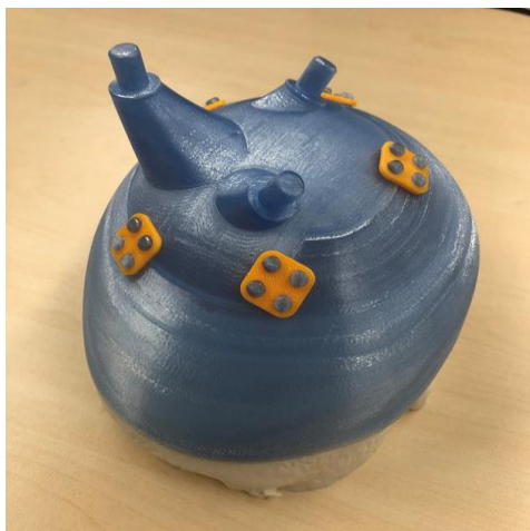
Figure 10: Patient customized magnetic focusing generator obtained by 3D printing according to the method proposed in this paper
