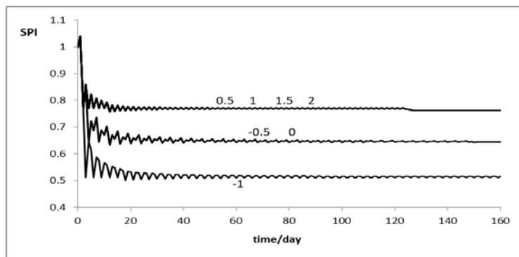
Figure. 8 Changes in the SPI of the project with changed alarm ratio
