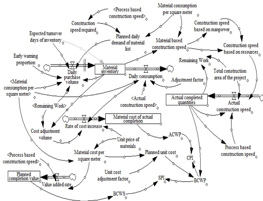
Figure. 2 Flow diagram of lean procurement system stack
