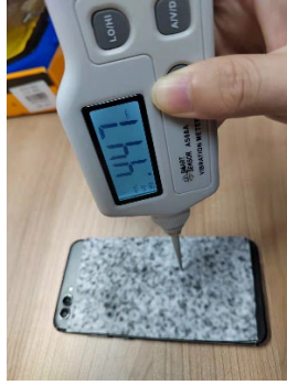
Figure 10: The vibration meter for mobile phone vibration test
