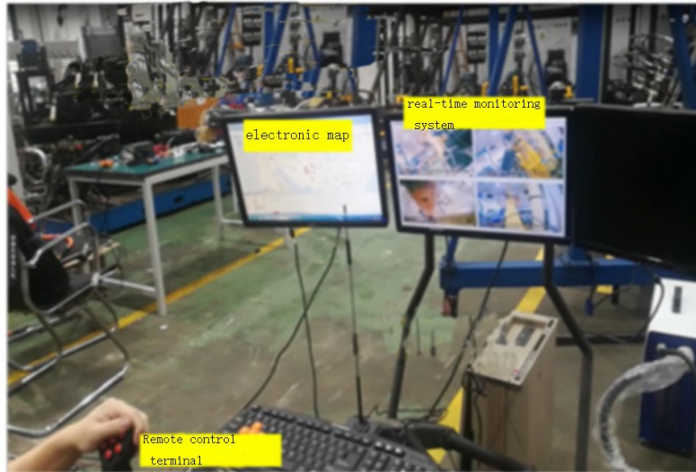
Figure 6: The real-time model of harvester and working information, and electronic map
