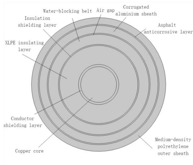
Figure 1: A crosslinked polyethylene cross-section model
