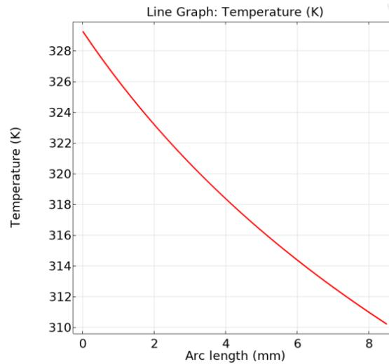
Figure 7: XLPE layer temperature curve
