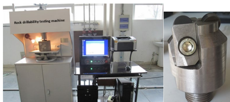
Figure 6: Rock drillability test equipment and micro-bit
