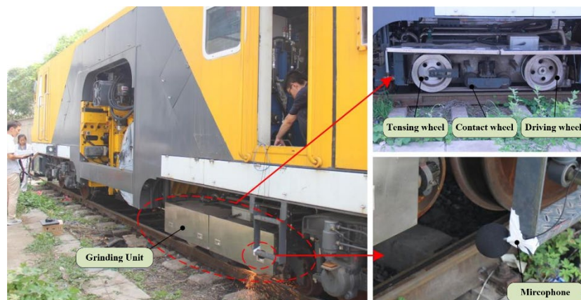
Figure 1: The rail abrasive belt grinding equipment.
