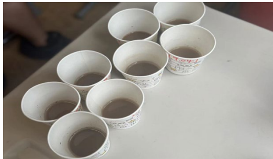
Figure 3: Samples are then allowed for standing precipitation
