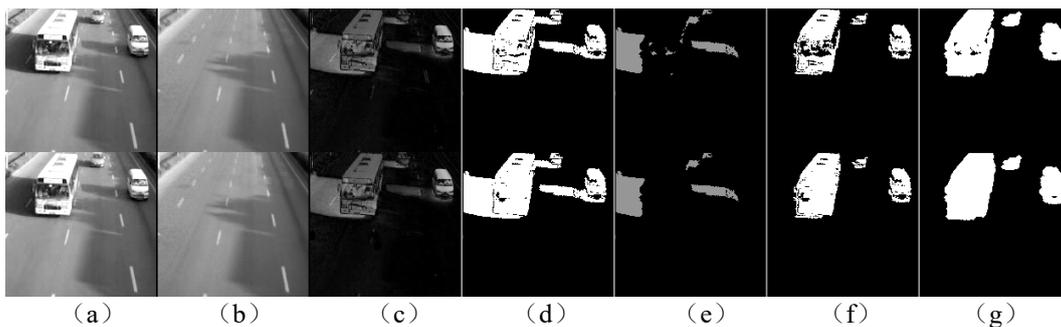
Figure 1 Shadow Removal Process of Moving Objects
