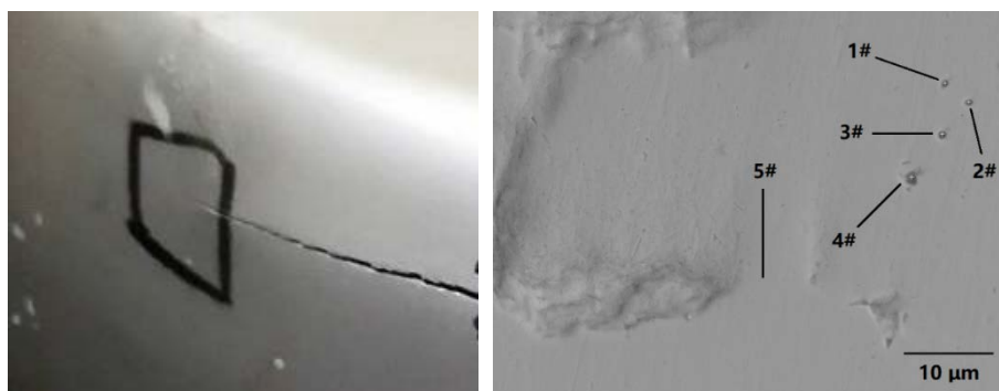
Figure. 6 Scanning Electron Microscope Analysis of Cracking Location of Stainless Steel Inner tank
