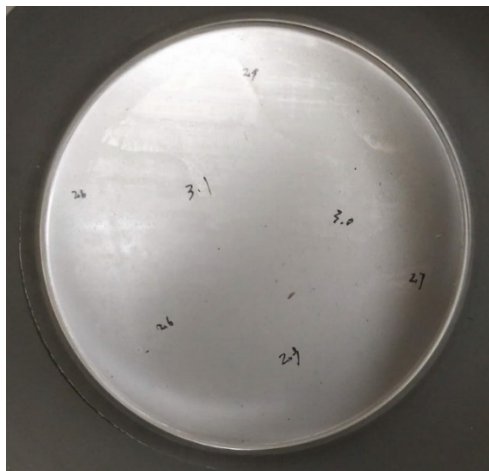
Figure. 2 Determination of martensite content in the bottom of stainless steel inner tank
