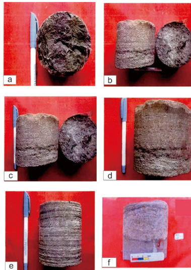
a. black mudstone, 144 well, 383m; b. gray fine sandstone, 7488 well, 412m; c. plate cross bedding, 144 well, 375m; d. trough cross bedding, e. parallel bedding, 6202 well, 427m; f. Scour surface, 423.76m, 966 well.
