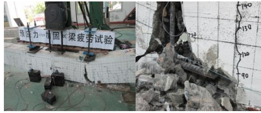
Figure 8: Failure mode of specimen A1
