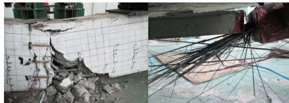
Figure 9: Failure mode of specimen B1
