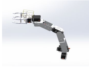
Figure 2: Six-degree-of-freedom tandem robotic arm
