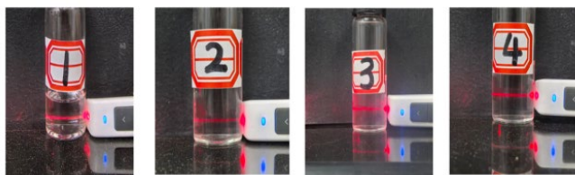
Figure 1. Schematic Diagram of the Tyndall Effect of Zirconia Sol
