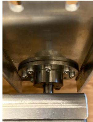
Figure. 6 Connection method of "knee" joint.
