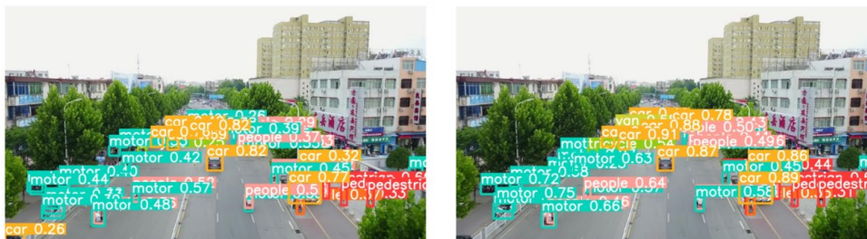
Figure 6: Comparison of detection effects on daytime road scenes between YOLOv5 (left) and the improved Model 4 of this paper (right).
