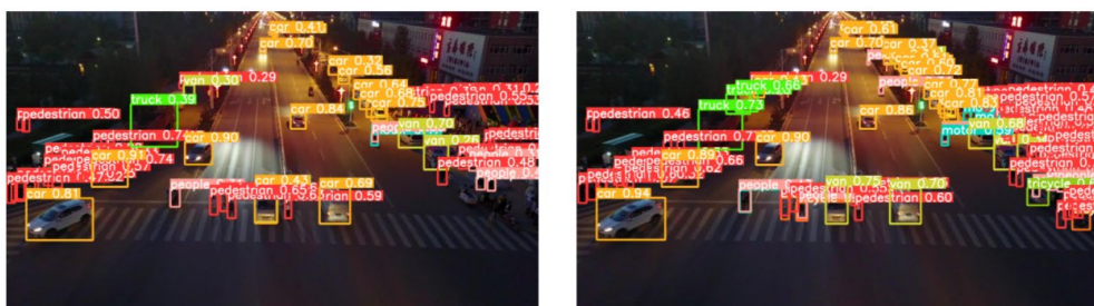
Figure 7: Comparison of detection effects in night-time dark scenes between YOLOv5 (left) and the improved Model 4 of this paper (right).
