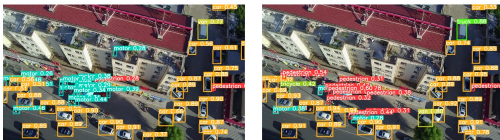
Figure 5: Comparison of detection effects in high-altitude shooting scenes between YOLOv5 (left) and the improved Model 4 of this paper (right).
