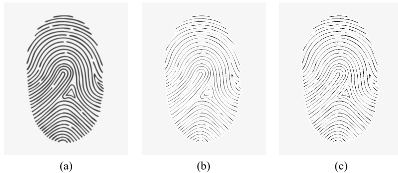
(a) Preprocessed image (b) direct thinning result (c) thinning result after adding orientation estimation
