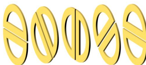
Figure 2 Schematic Diagram of Coupling Mechanism in Multi-Relay Wireless Power Transfer System
