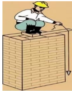
Figure 10: Worker with Plumb Line
