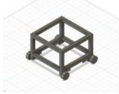
Figure 6: The 3D model of the car's body and chassis.
