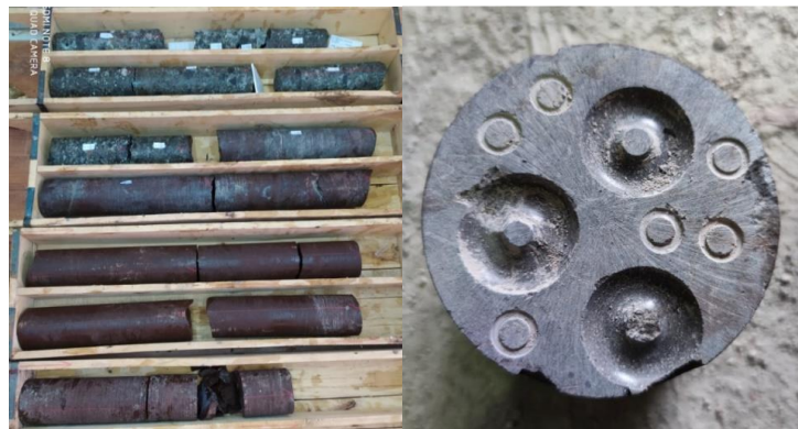
(a) Straturn drilling core (b) Drillability measurement
