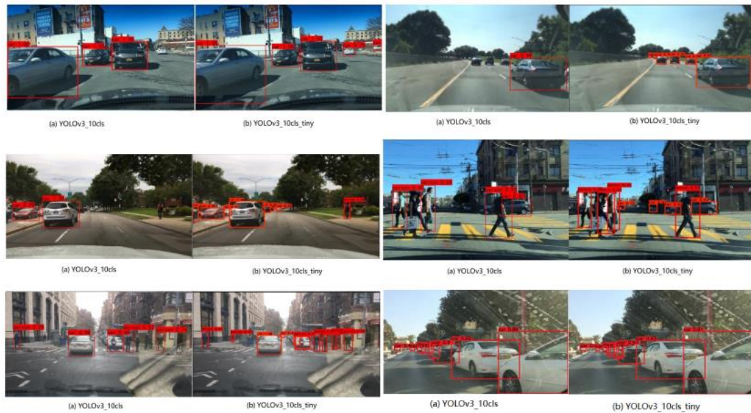
Figure 4: Comparison of YOLOv3_10cls and YOLOv3_10cls_tiny detection results
