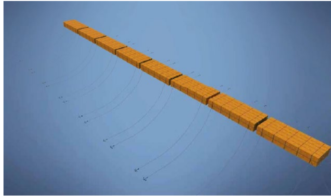
Figure 7: Layout of rectangular type cost-effective floating breakwater[37]
