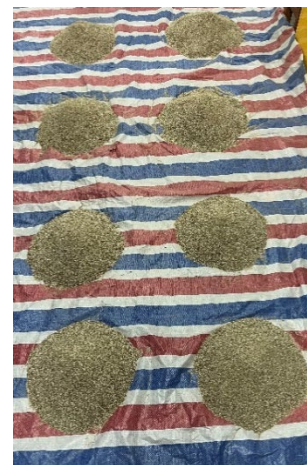
Fig.4 Sand box structure diagram Fig.5 Sand samples are taken by four-point method
