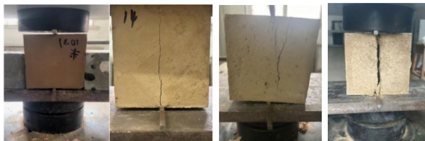
(a) Specimen placement (b) Crack formation (c) Through crack (d) Specimen failure
