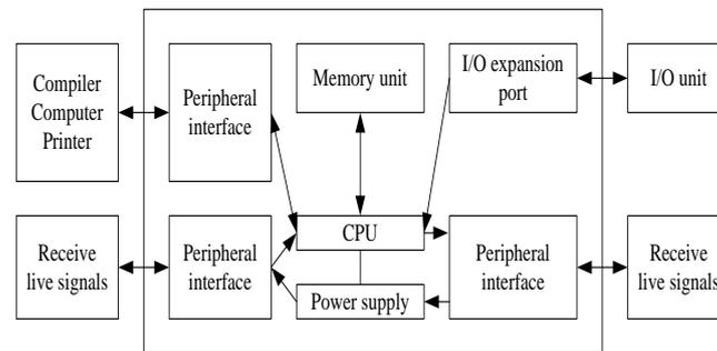
Figure 1: Basic Structure of PLC
