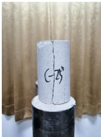
Fig.5 Experimental Phenomena of Triaxial Compression of White Sandstone Specimen
