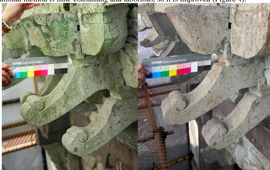
Figure 4: Comparison of chemical material before and after application of dodecyl dimethyl benzyl ammonium chloride
