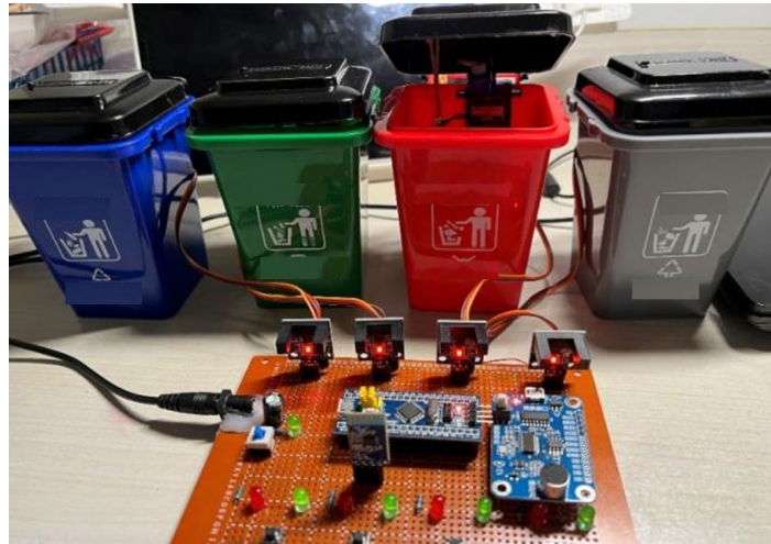
Figure 9: Voice recognition automatic control of physical test diagram
