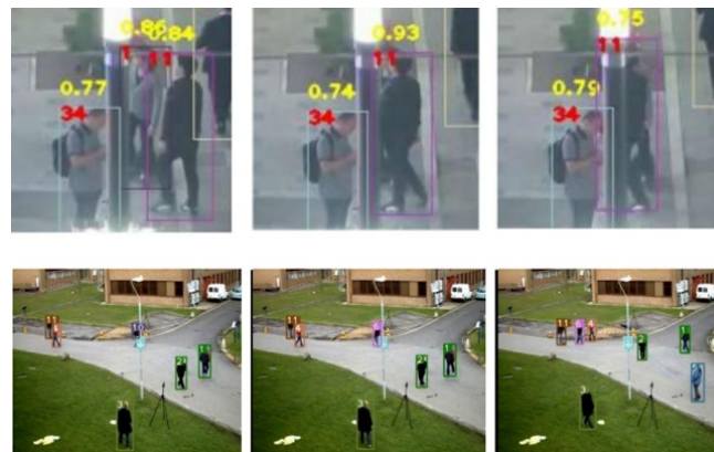
Figure 4: CenterNet tracking results with occlusions
